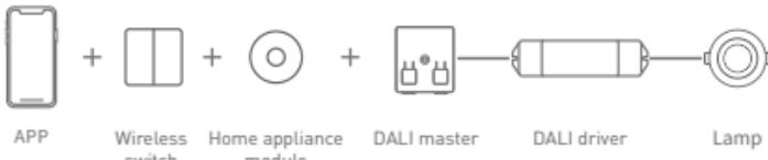
4. Visual control + Traditional dimming panel and remote controller control.
