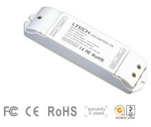
LED Power Repeater is suitable for all of our company's power-output style controllers' power expansion, it accepts PWM control, the control quantity of LED lights would be twice as much by adding one more power repeater, unlimited quantity of power repeater to be connected theoretically.
