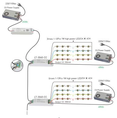
3.2 Repeaters connected to DMX constant current decoder:
