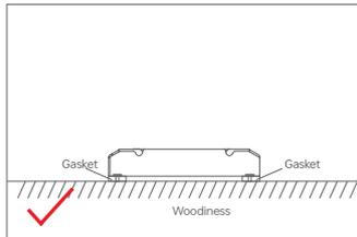
Do not fix the product tightly against the wooden board with screws. Please add a washer  $\geq 7\text{mm}$  thick under the mounting screws to leave a gap for effective heat dissipation, so as to avoid affecting the heat dissipation and service life of the product.
