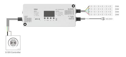
3.Connect two color temperature lights simultaneously, with each controller managing one light. Set the dimming mode to "CT" in the NFC Lighting app.
