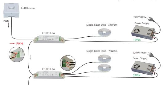
Power repeater connected to LED dimming driver:
