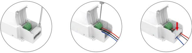
Use a screwdriver to pry up the protective housing at the edge of the wire fixing board. Then connect to the wires as the diagram shows and press down the wire fixing board.
