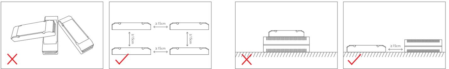
Please do not stack the products. The distance between two products should be  $\geq 15\text{cm}$  so as not to affect heat dissipation or the lifetime of the products.
