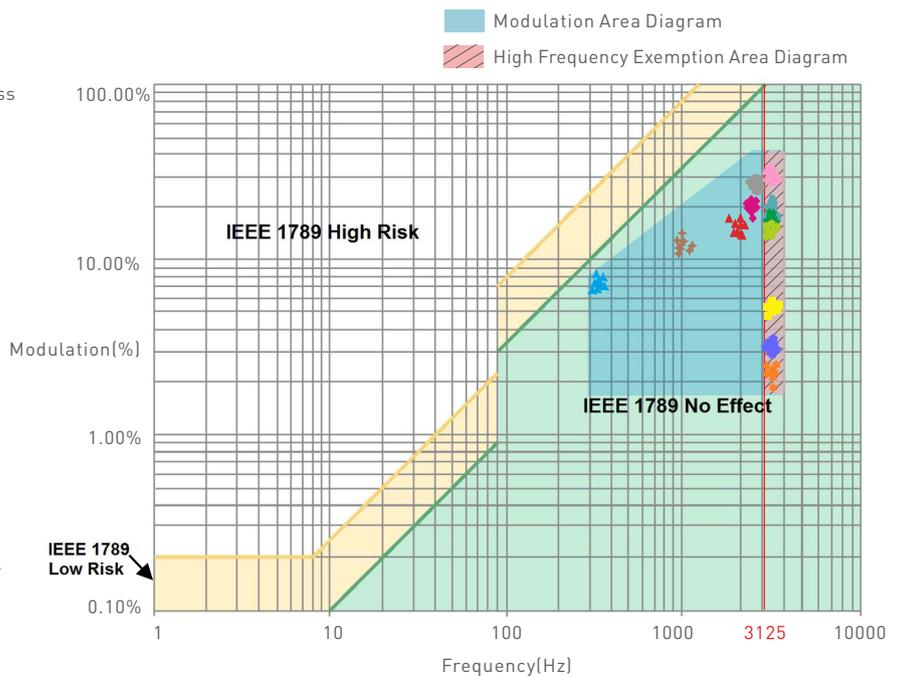
Marks in the right chart were tested results of different current ranges. The output frequency is 0Hz in 100% brightness and its corresponding modulation is 0%, which could not be shown in the right chart.
