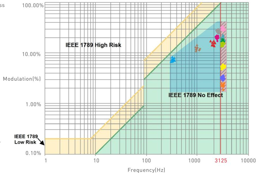
Marks in the right chart were tested results of different current ranges. The output frequency is 0Hz in 100% brightness and its corresponding modulation is 0%, which could not be shown in the right chart.
