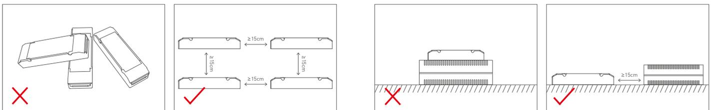
Please do not stack the products. The distance between two products should be  $\geq 15\text{cm}$  so as not to affect heat dissipation and the lifespan of the products.
