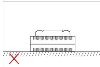
Please not place the products on power supplies. The distance between the product and the power supplies should be  $\geq 15\text{cm}$  so as not to affect heat dissipation or shorten the lifetime of the products.
