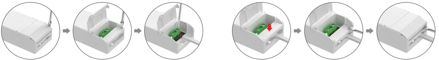
1. Put the head of a screwdriver on the side of the housing to pry up both the protective cover and wire fixing board. Then remove the wire fixing board and connect to the wires as wiring diagram shows.
