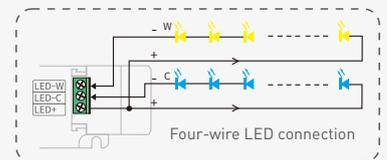
\* Adopting constant power program design, it keeps the same brightness in color temperature dimming, and twice the rated power load can be connected.
