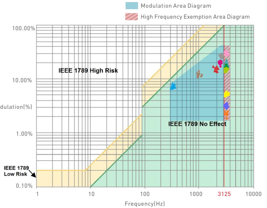
Marks in the right chart were tested results of different current ranges. The output frequency is 0Hz in 100% brightness and its corresponding modulation is 0%, which could not be shown in the right chart.
