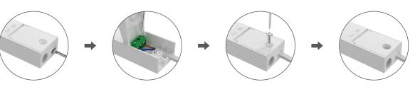
1.Put the head of the screwdriver at the cable entry to pry up the protective cover, then connect the wires as the wiring diagram shown
